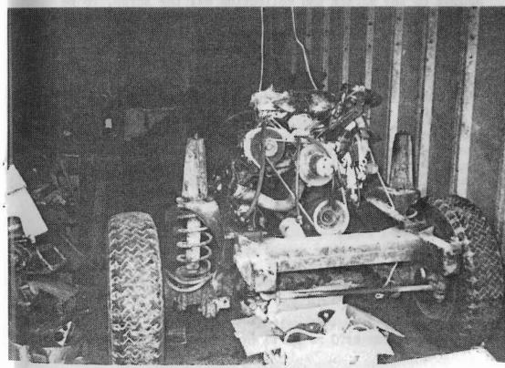
Back to the rolling chassis, the next job being removing the engine and gearbox unit in one piece. This was duly carried out and the unit was loaded onto my friend's box trailer, which was to be stored in his garage until needed, Thank you John.
